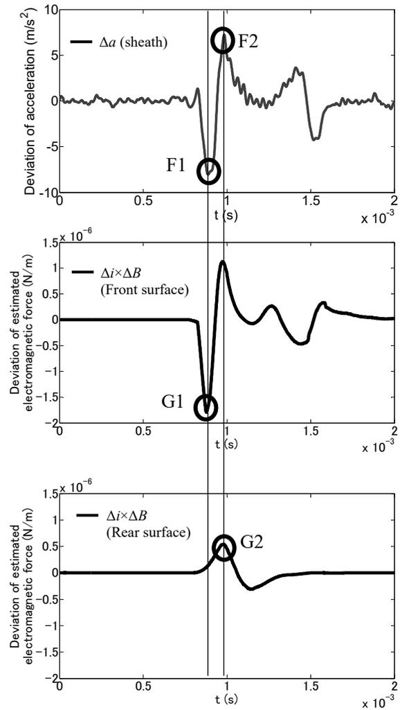
**Fig. 4 Relation between elastic and electromagnetic responses of a sheath and PC bar**
