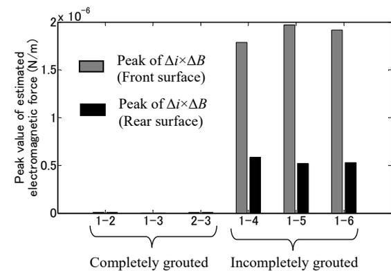
**Fig. 5 Estimation results (peak value of estimated electromagnetic force)**
