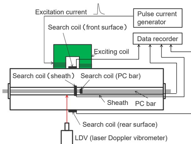
Fig. 1 Configuration of the measurement system
