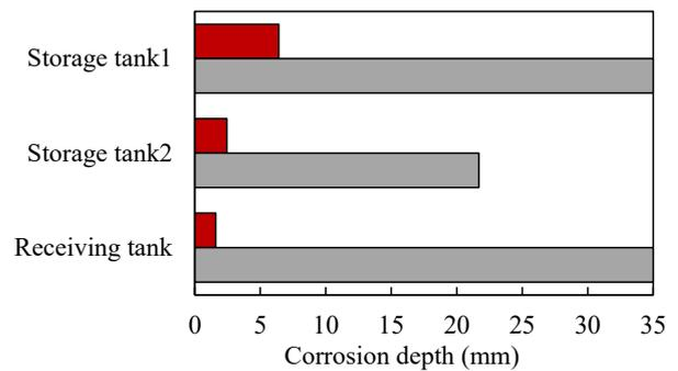
**Fig. 3 Resistance to sulfuric acid by exposure tests in sewage facilities**
