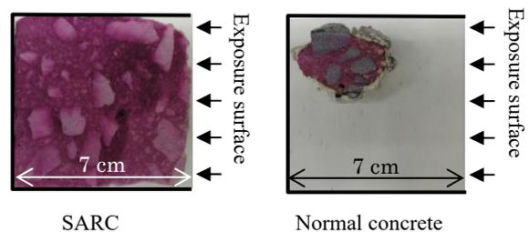
**Photo 1 Resistance to sulfuric acid by exposure test in a sewage facility (storage tank 1)**
