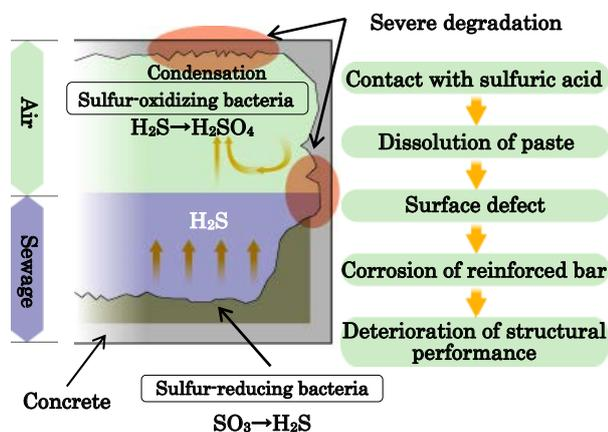
Fig. 1 Degradation of concrete in sewage facilities by sulfuric acid
