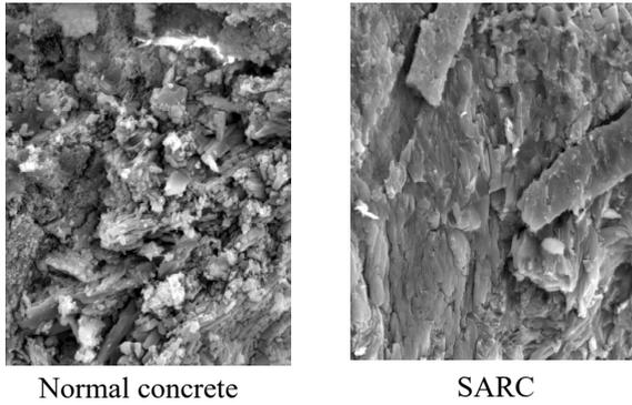
Photo 2 Secondary electron images of surface gypsum after immersion in sulfuric acid
