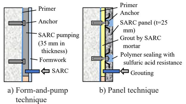
Fig. 5 Schematic diagrams of repair work
