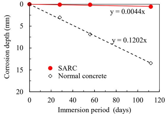
**Fig. 2 Resistance to sulfuric acid by immersion test**
