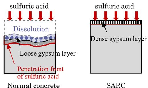
**Fig. 4 Mechanism of sulfuric acid resistance**
