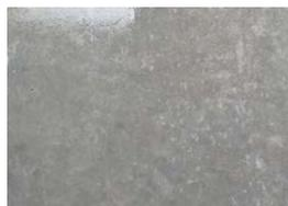
Sheet curing; area ratio of surface air voids = 0.06%
