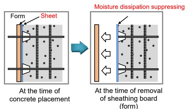
Fig. 2 Overview of sheet curing method
