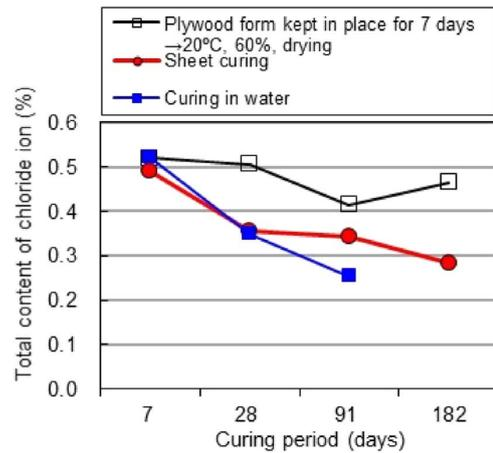
Fig. 4 Results of salt penetration tests<sup>[1]</sup>
