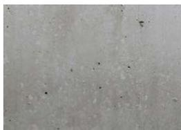
Plywood; area ratio of surface air voids = 0.45%
