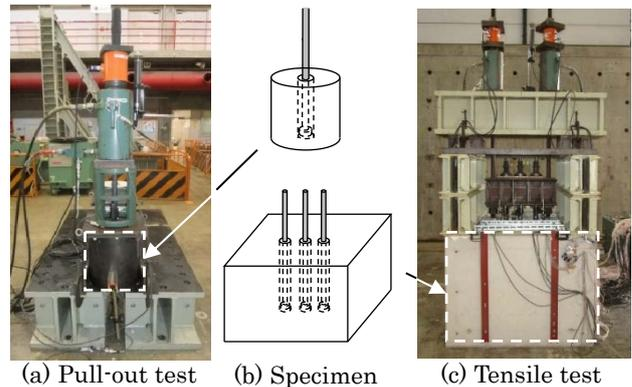
Fig. 4 Setup of experiments
