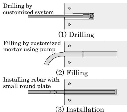
Fig. 2 Outline of anchor installation system
