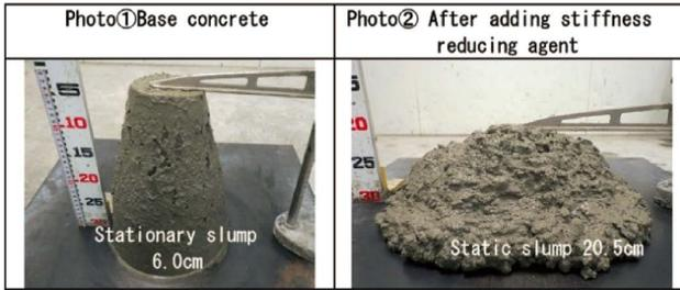
Fig. 1 Comparison of static slump test results
