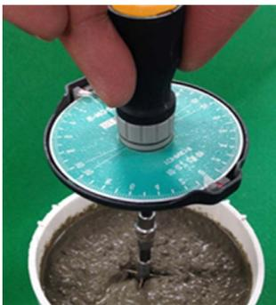
Fig. 2 Vane shear test
