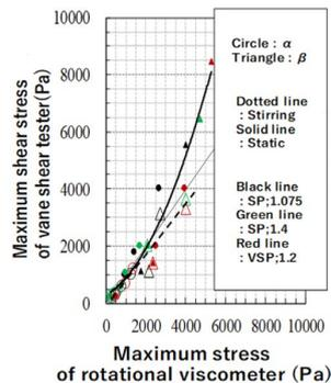
Fig. 3 Comparison of results from rotational viscometer and vane shear tester
