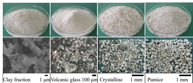
**Fig. 2 Four types of mineral after sorting<sup>[1]</sup>**
