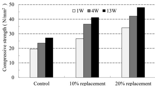
Fig. 4 Compressive strength tests (W/B=0.61)<sup>[1]</sup>
