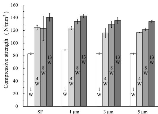
Fig. 3 Compressive strength tests (W/B=0.2)<sup>[1]</sup>
