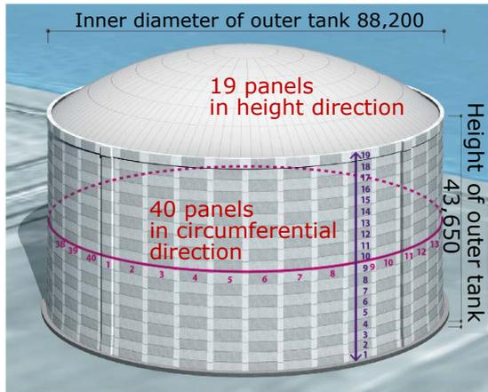
Fig. 4 Arrangement of precast panels (unit: mm)
