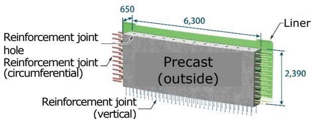
Fig. 5 Image of precast panel (unit: mm)
