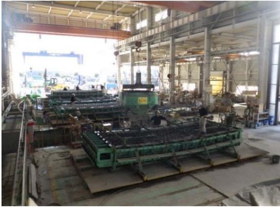
**Fig. 8 Manufacturing of precast panels**
