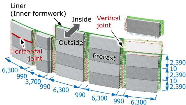
Fig. 6 Joints of precast panels (unit: mm)
