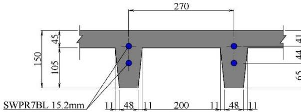
**Fig. 8 Enlarged sectional view of ribs in the transverse direction**
