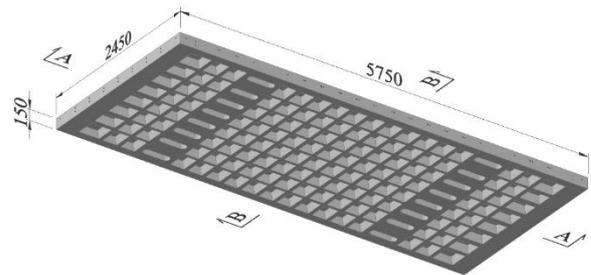
**Fig. 4 Conceptual diagram of a standard panel**
