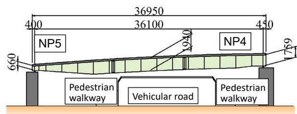
Fig. 1 Side view of the Shinanobashi Rampway Bridge
