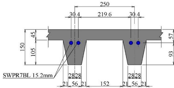
**Fig. 7 Enlarged sectional view of ribs in the longitudinal direction**
