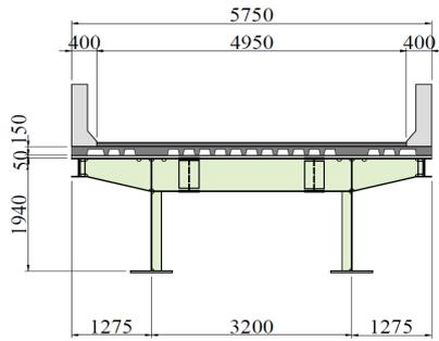
**Fig. 2 Sectional view of the Shinanobashi Rampway Bridge**
