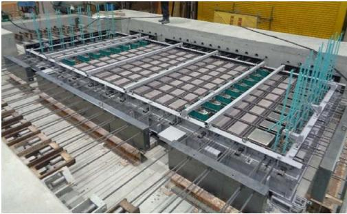
Fig. 10 Status after tensioning of PC steel bars
