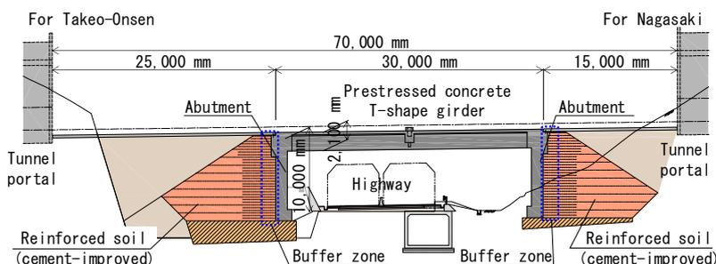
Fig. 2 General view of the GRS integrated bridge with PC girders (Genshu over-road bridge)
