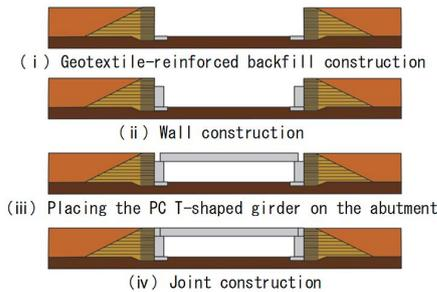
Fig. 3 Construction process of the GRS integrated bridge
