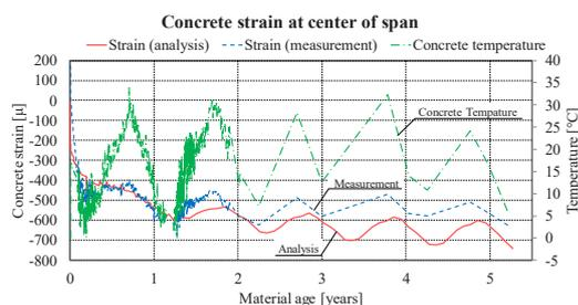
Fig. 5 Concrete strain at the center of the span
