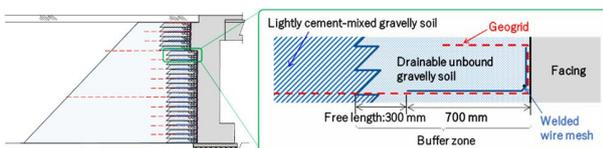
Fig. 4 Buffer zone of the GRS integrated bridge
