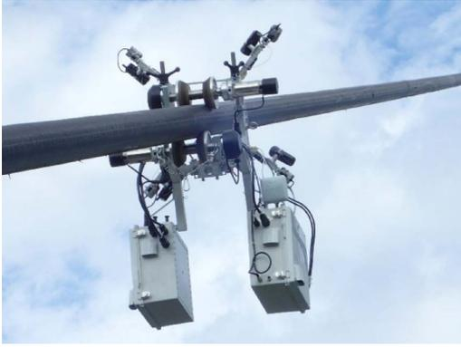
Fig. 3 Self-propelled stay-cable inspection device
