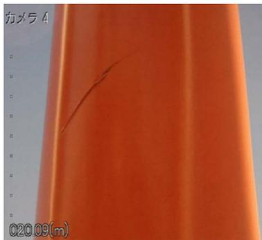
Fig. 4 Image of a protection pipe taken by the device
