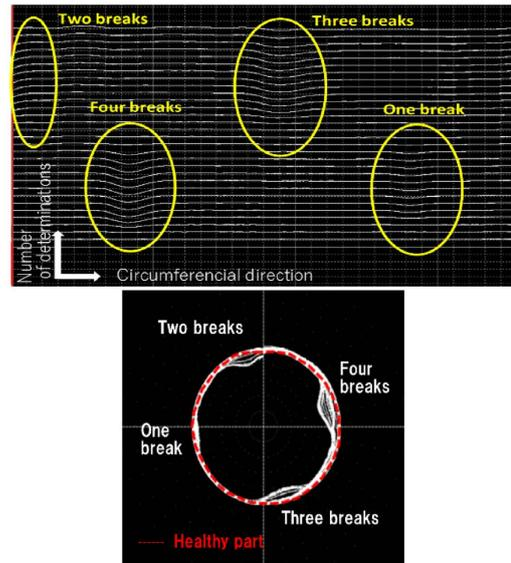
Fig. 5 Line and circular waveform detected by eddy current test
