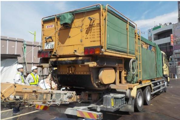
Fig. 9 Jet concrete mixer truck
