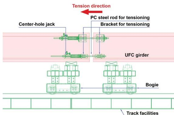
Fig. 5 Joining equipment
