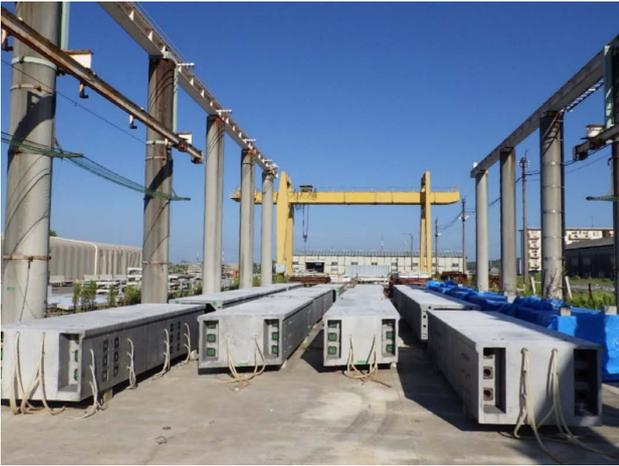
Fig. 4 Fabrication of UFC segments
