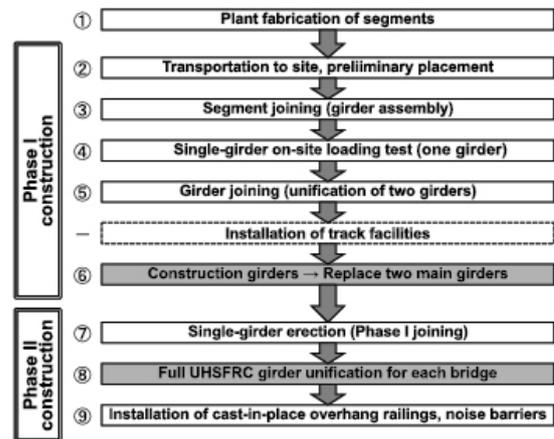
Fig. 3 Construction flow
