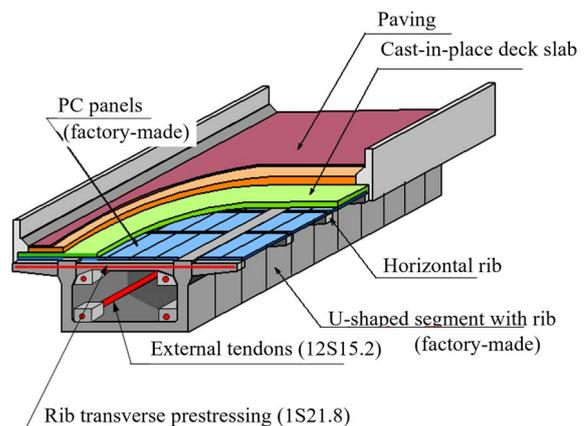
**Fig. 3 Overview of the box structure**
