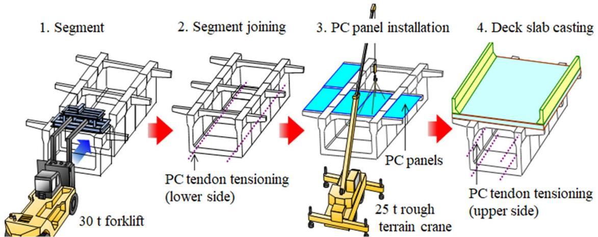
Fig. 4 Box culvert construction processes
