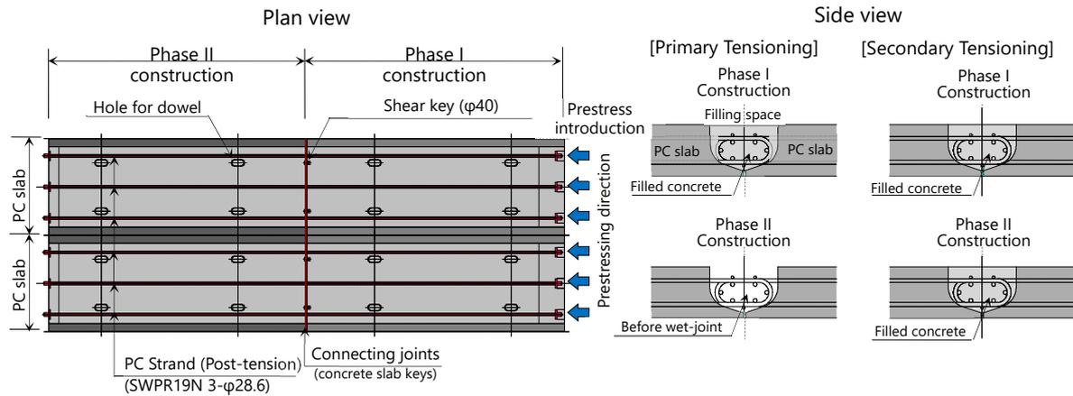
Fig. 5 Conditions of connecting joints at time of introducing prestress for each phase
