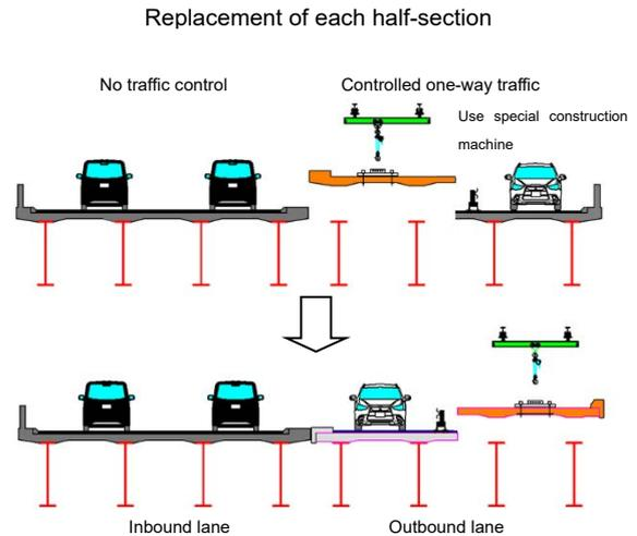
Fig. 3 Example of replacing each half-section
