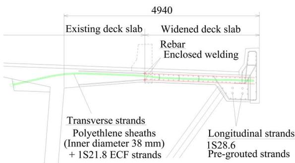
Fig. 5 Detailed view of widened deck slab section
