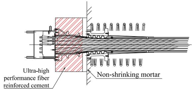
Fig. 6 Anchoring device (UHPFRC)
