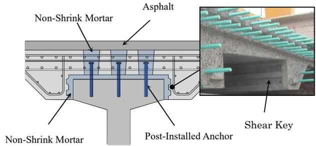
Fig. 4 Details of joints between the PCa panels and PC girders
