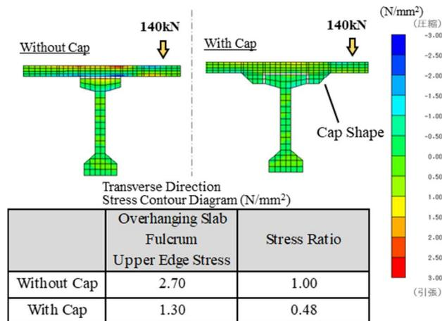
Fig. 2 Cap shape effect (stress reduction)
