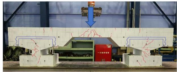
Fig. 5 Full-scale structural performance verification experiment (load transfer verification)
