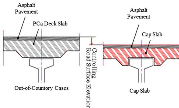
Fig. 3 Cap shape effect (deck level reduction)
