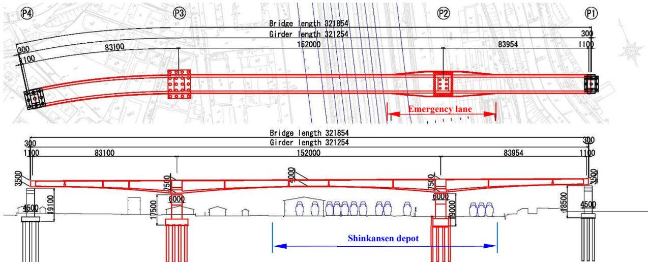
Fig. 3 Overview of Yaga Overpass Bridge
