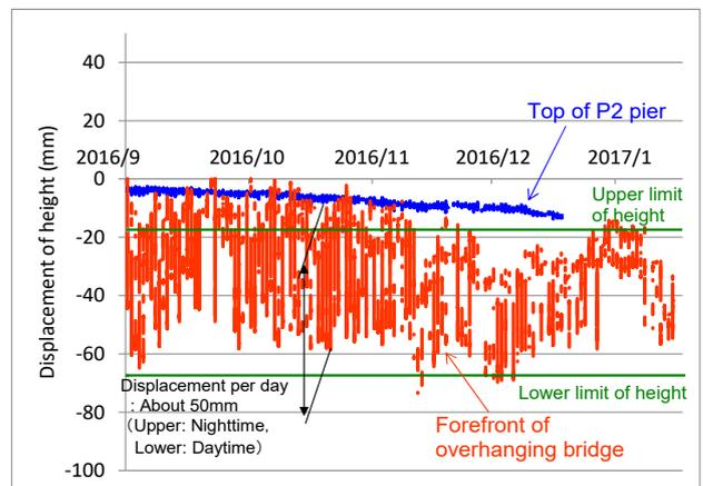
Fig. 9 Elevation change at the overhang tip superstructure heights
