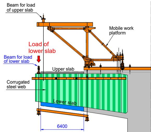
Fig. 6 Load-supporting mechanism of the lower slab concrete
