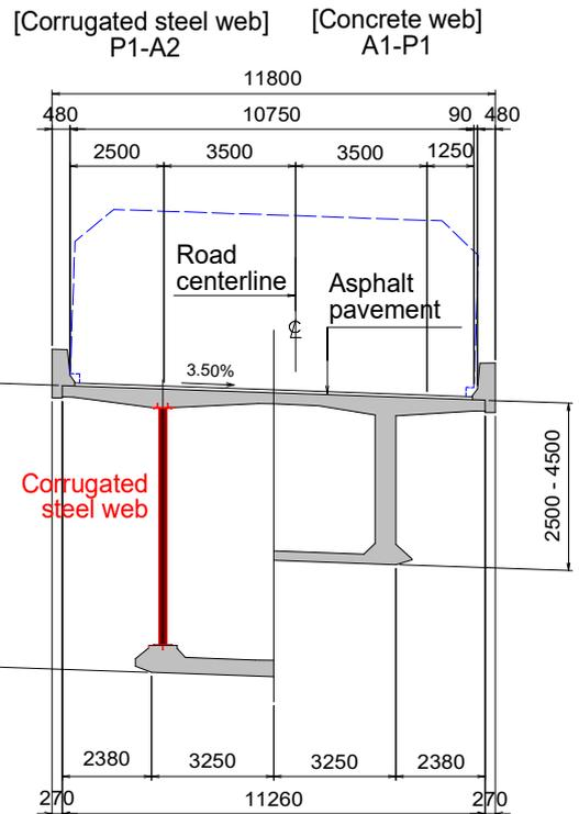
Fig. 4 Standard section of the superstructure of the outbound lane
