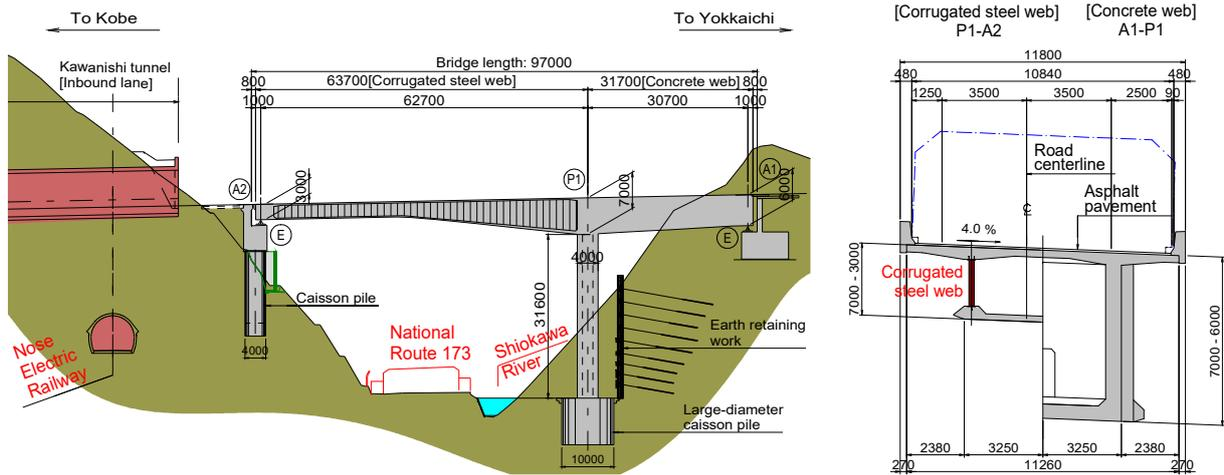
Fig. 2 Overall diagram and standard section of the superstructure of the inbound lane
