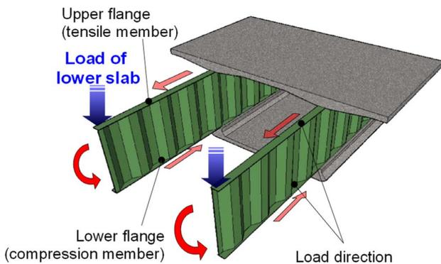
Fig. 5 Load-carrying mechanism lower slab
