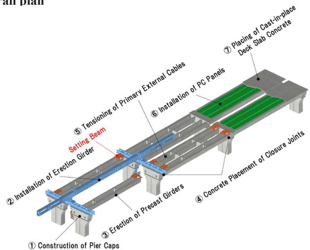
Fig. 3 Construction procedure
