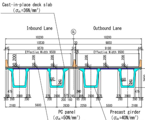
Fig. 2 Typical cross section
