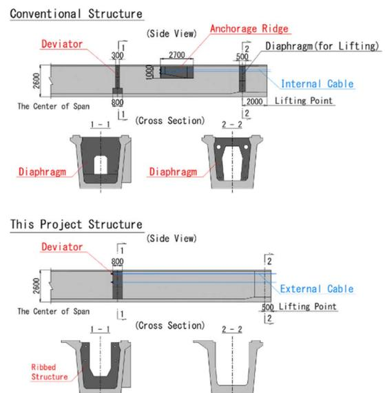
Fig. 7 Comparison of precast girder structures
