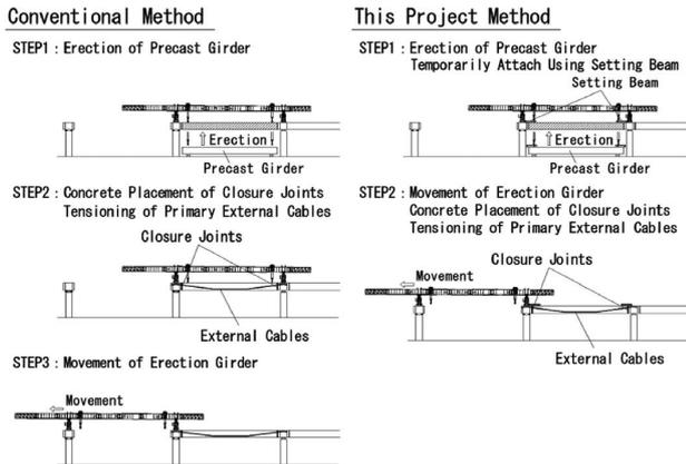
Fig. 9 Comparison of erection methods
