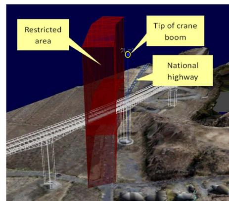
Fig. 7 GNSS crane monitoring system
