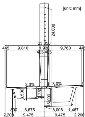
Fig. 2 Cross section
