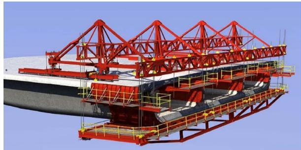
Fig. 11 3D drawing of form traveller
