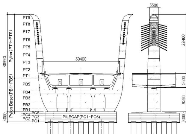
Fig. 4 General view of pylon and pier head (with view of concrete casting layer)
