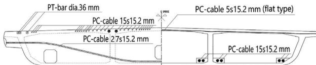
Fig. 8 Arrangement of prestressing steel
