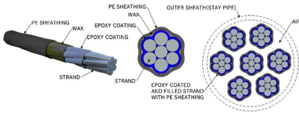
Fig. 12 Four-layer anticorrosion specification
