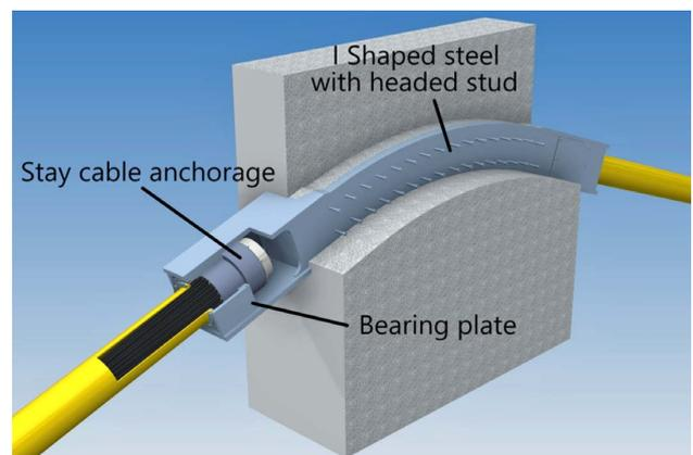
Fig. 6 Stay cable anchorage-type saddle
