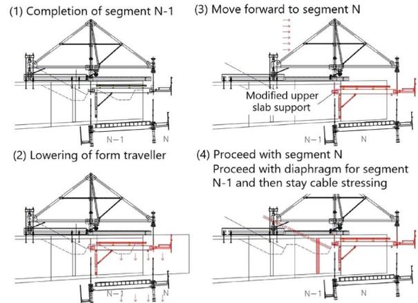
Fig. 9 Sequence of stay cables and diaphragms
