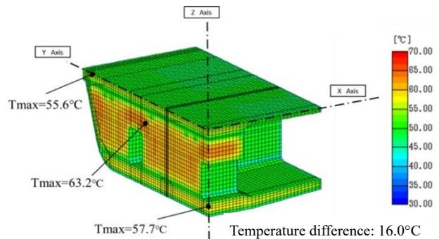
Fig. 5 Maximum temperature distribution of the transverse girder after pipe cooling (1/4 model of pier head)
