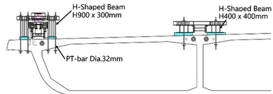
Fig. 14 Displacement restraint of main girder
