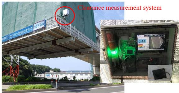
Fig. 6 Clearance measurement system
