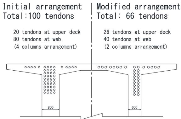
Fig. 6 Comparison of maximum tendon arrangements
