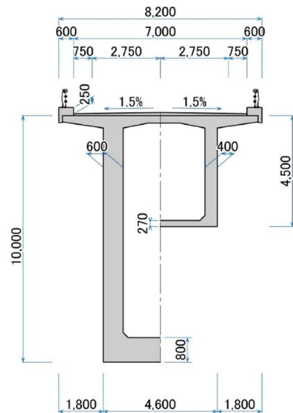
Fig. 5 Cross section of main girder
