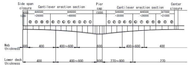
Fig. 7 Comparison of block segments
