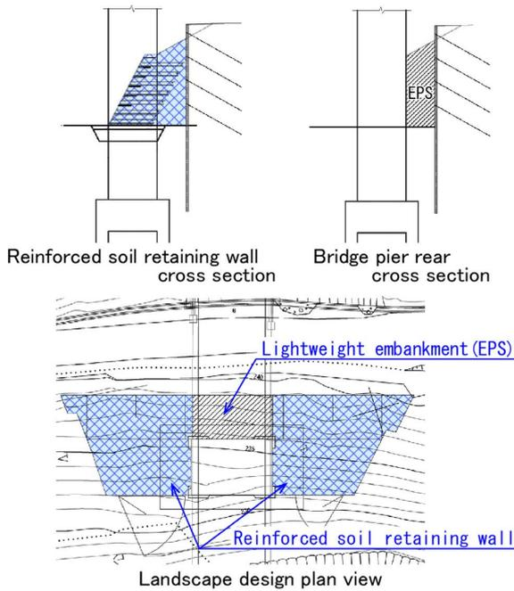
Fig. 3 Use of lightweight embankment
