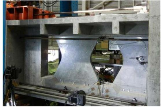
Fig. 2 Testing for shear capacity
