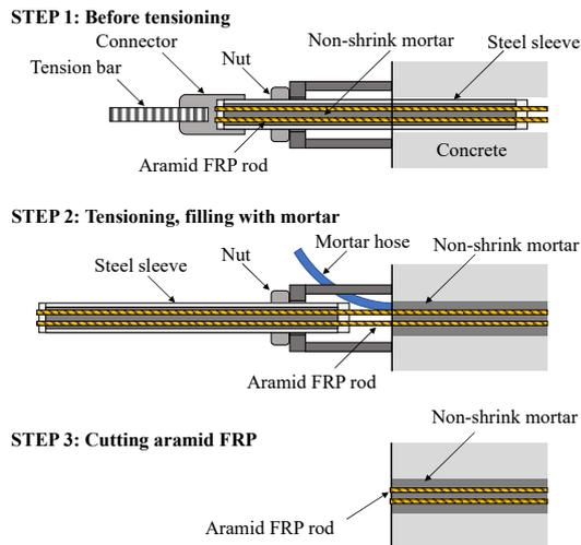
Fig. 8 Tensioning procedure for external cables
