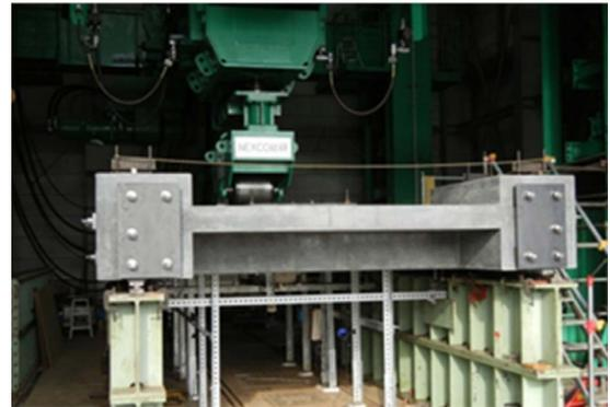
Fig. 3 Wheel load running test
