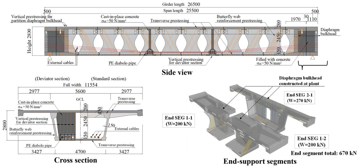
Fig. 5 Structural overview of the Bessodani Bridge
