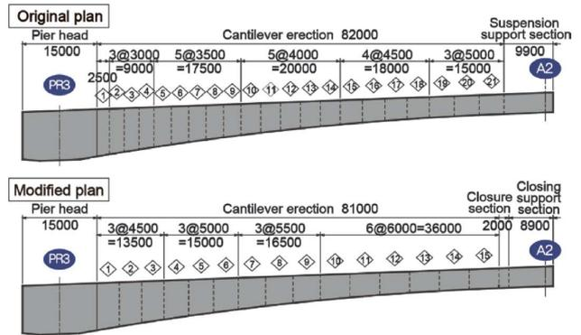
Fig. 7 Comparison of main girder blocks (PR3 side)
