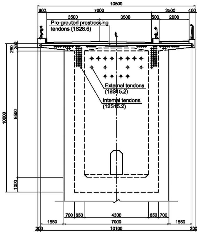
Fig. 2 Cross section at pier head
