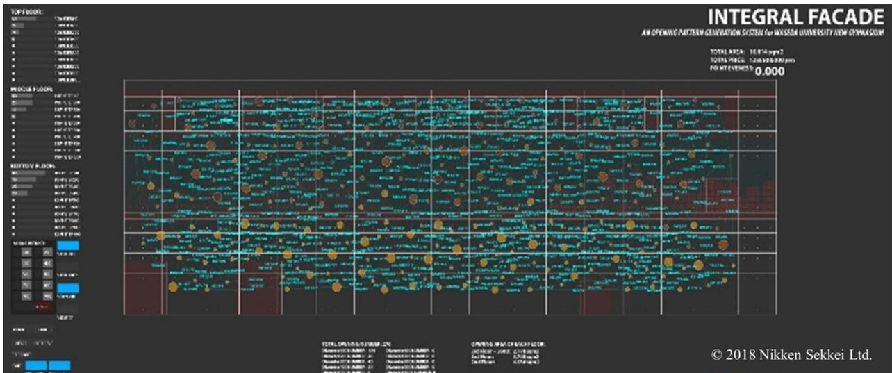
Fig. 3 Program for calculating the layout of the circular openings
