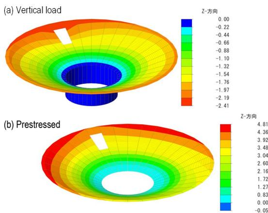
Fig. 5 Cofun A: vertical displacement (mm)
