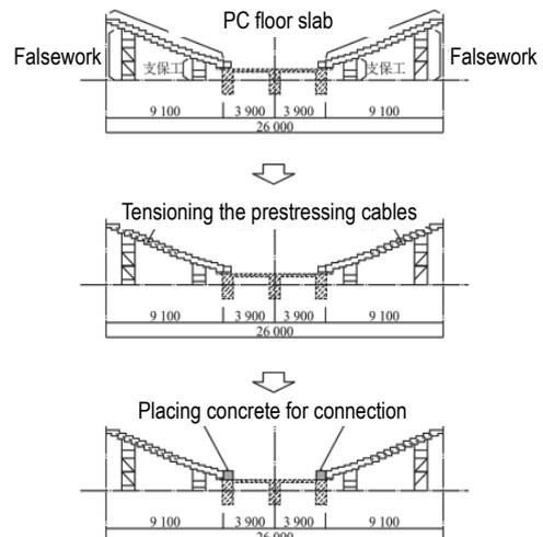
Fig. 9 Construction of Cofun A
