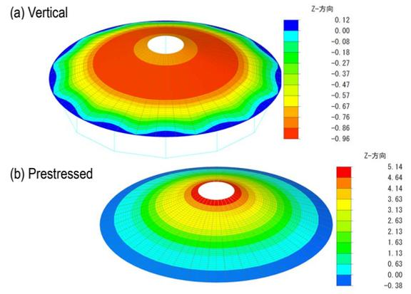
Fig. 6 Cofun C: edge compressive stress (N/mm<sup>2</sup>)
