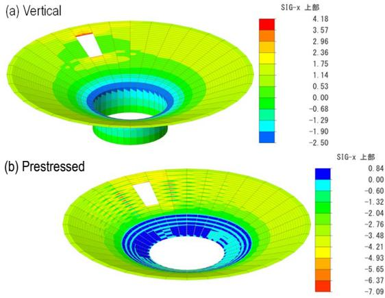
Fig. 4 Cofun A: edge compressive stress (N/mm<sup>2</sup>)
