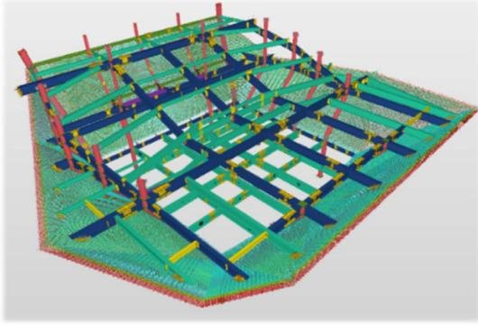
**Fig. 8 Confirmation of interference with steel frame by Solibri**
