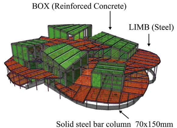
Fig. 4 Structural analysis model
