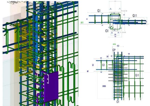
**Fig. 9 Step 1: 3D model for rebar**
