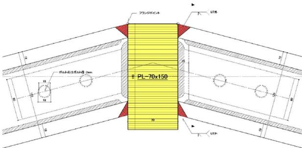
**Fig. 8 Joint detail**
