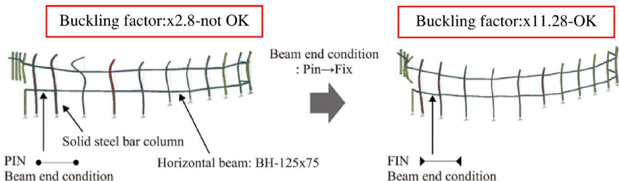
Fig. 6 Results of buckling analysis
