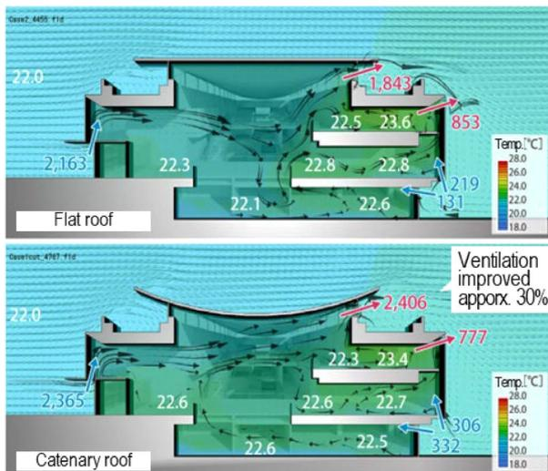
Fig. 4 Effect of roof shape on ventilation
