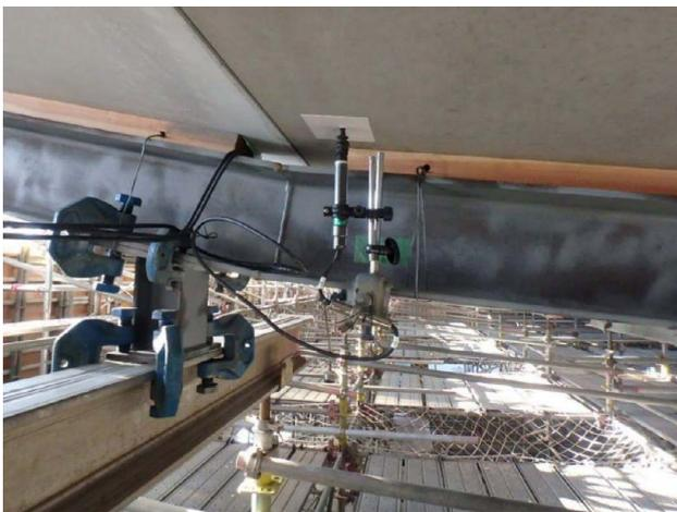
Fig. 13 High-precision displacement transducer
