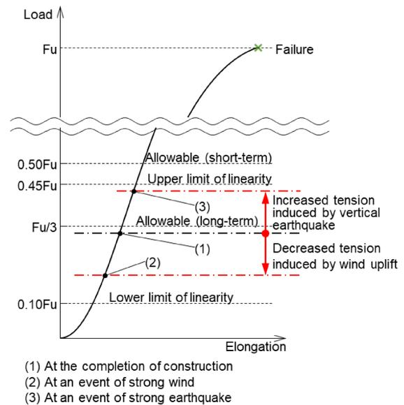
Fig. 5 Load-elongation model of cables
