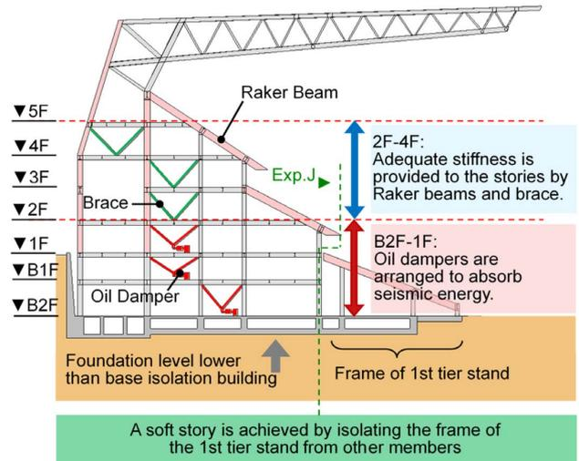
Fig. 6 Response-controlled structure by means of a soft-first-story system
