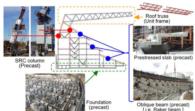
Fig. 7 Unitization and prefabrication of members
