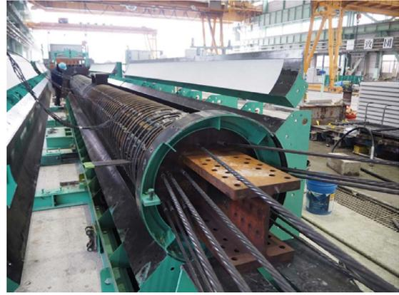
Fig. 11 SRC column manufactured at the precast factory
