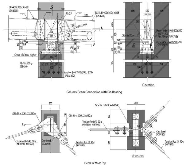
Fig. 7 Joint of reinforced concrete and steel elements
