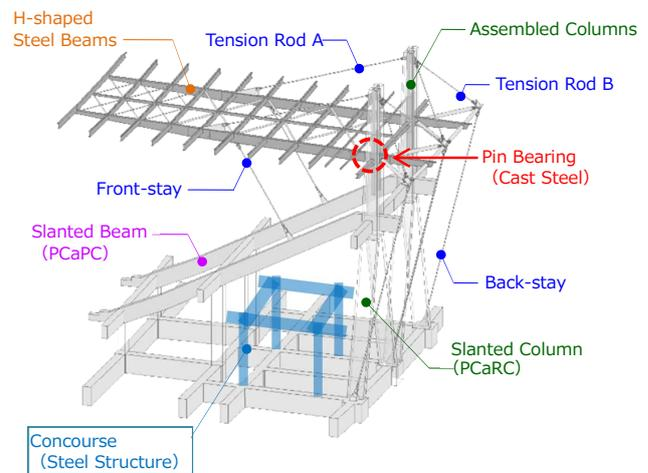
Fig. 4 Basic structural concept
