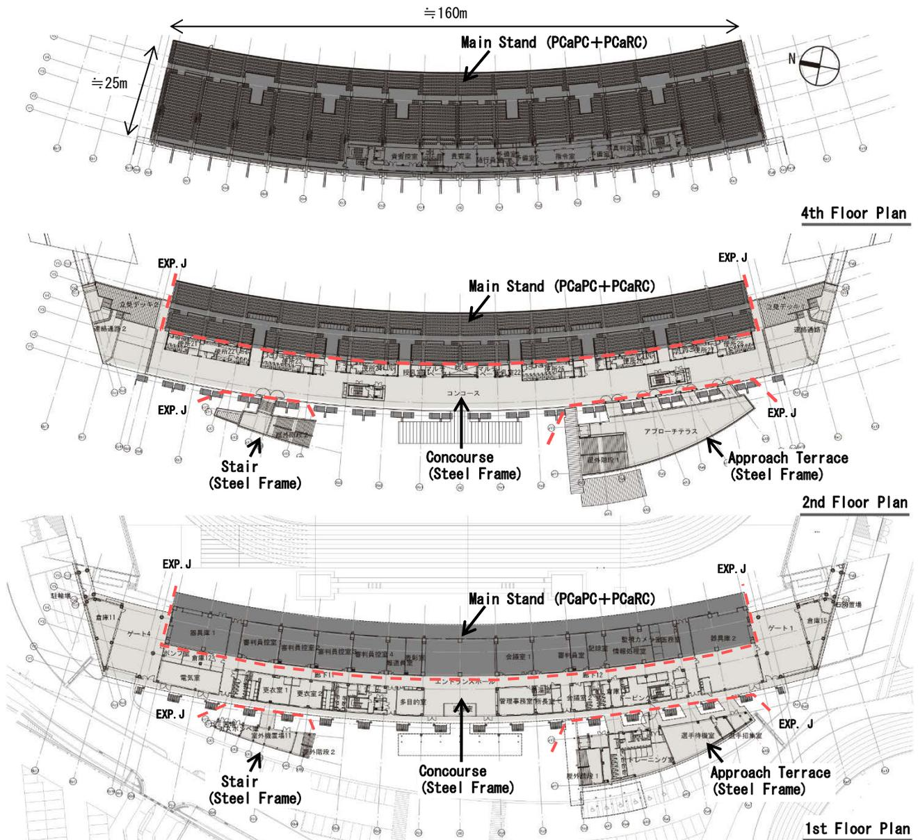
Fig. 5 Floor plan
