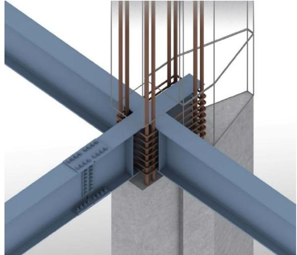
Fig. 5 Beam-to-column connection
