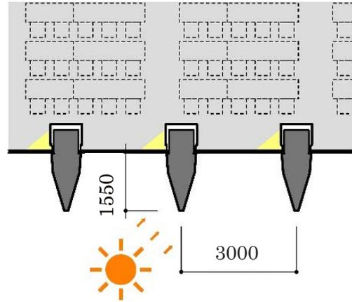
Fig. 8 Column shape with added sunlight shielding effect
