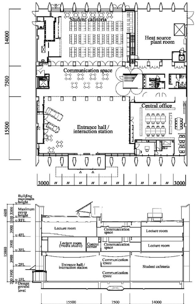
Fig. 2 First-floor plan and cross-section
