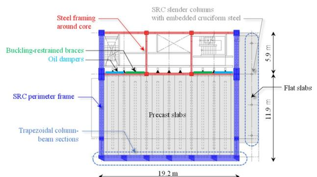
**Fig. 5 Typical floor plan + structural labels**
