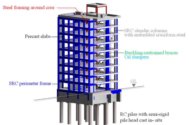
**Fig. 4 Structural framing 3D model**
