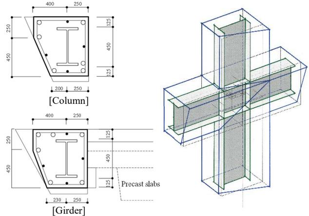
Fig. 8 Trapezoidal columns & beams + SRC concept
