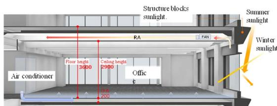
**Fig. 3 Section view through the office area**
