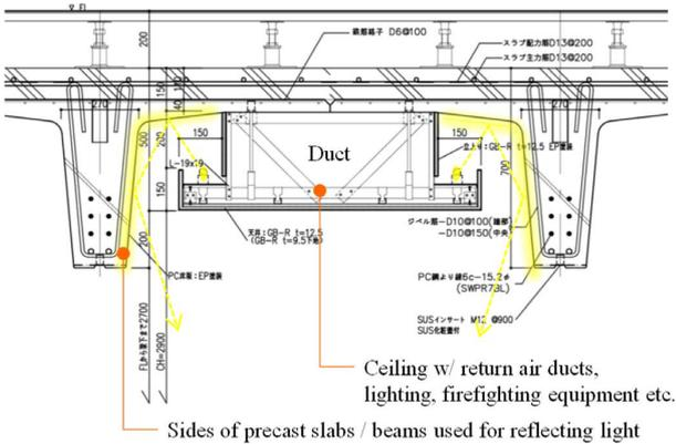
Fig. 6 ST floor slab and duct ceiling
