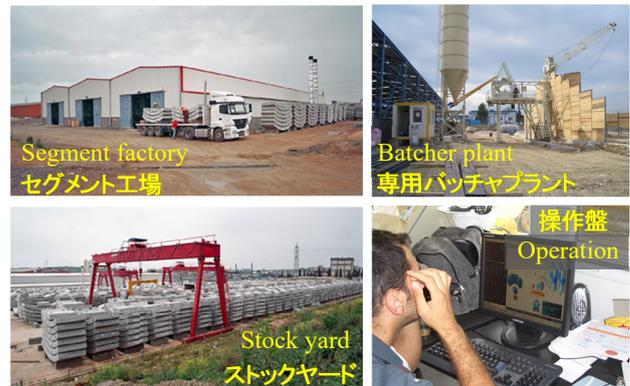
Fig.4 Segment factory for TBM tunnel
