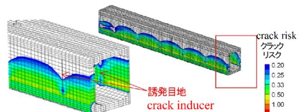
Fig.2 Results of 3D temperature and stress analyses
