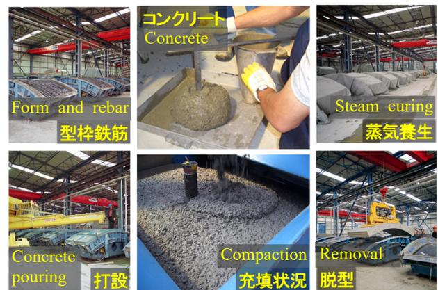
Fig.5 Segment production process
