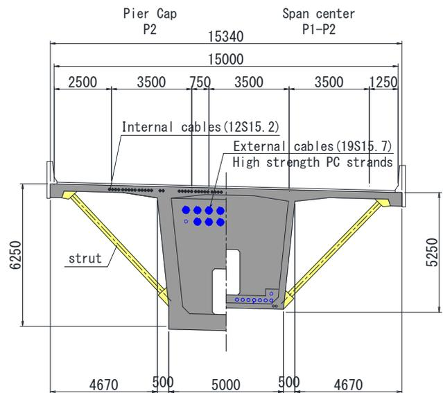
**Fig.3 Main-girder cross section**
