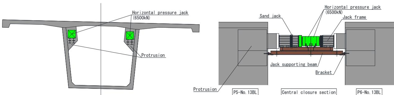
Fig.6 Detailed diagram of horizontal-loading device
