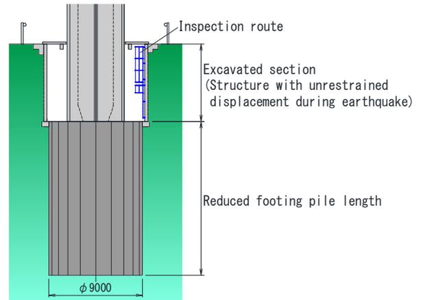
Fig.4 Excavated pier
