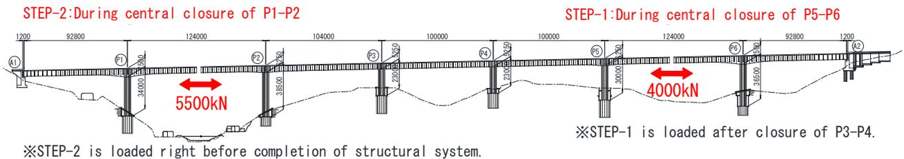
Fig.5 Horizontal-loading location and order
