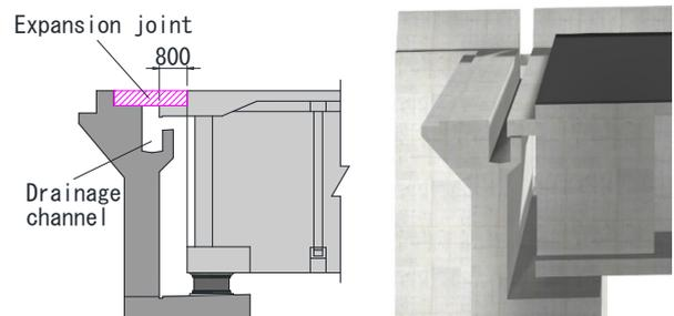
Fig.7 Setback joint structure
