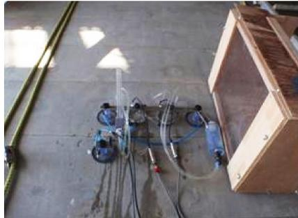
**Fig.9 Measure water-permeability**
