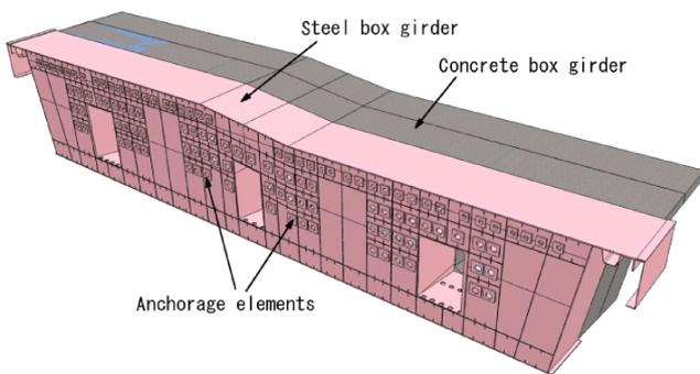
Fig.3 Joint section (P2 side)
