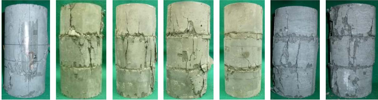
UFC 単体 No. 5 (t=2.4mm) No. 6 (t=5mm) No. 7 (t=8mm) No. 8 (t=12mm) No. 9 (t=1.2mm) No. 10
