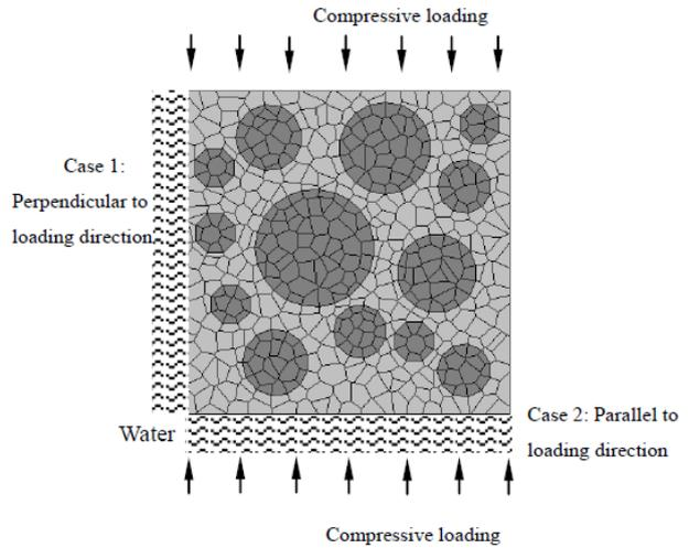
Fig. 4 Geometry of the meshed concrete specimen and analysis conditions under compression
