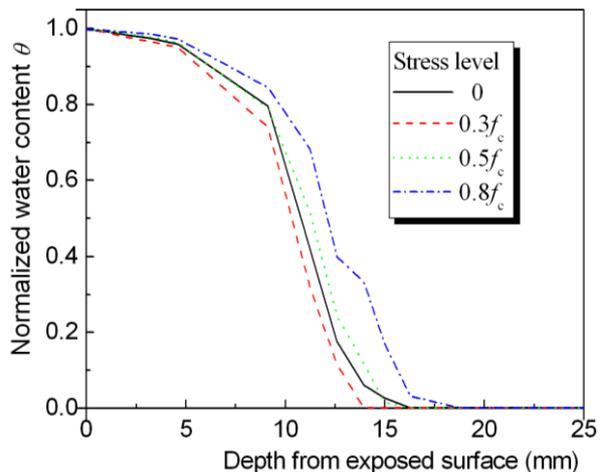
Fig. 8 Water content distribution under different compressive stress levels
