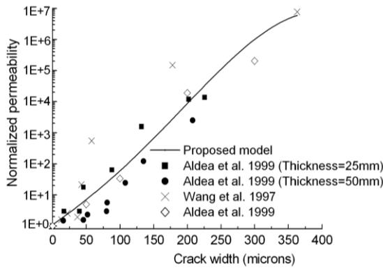
Fig. 3 Relationship between normalized permeability and crack width
