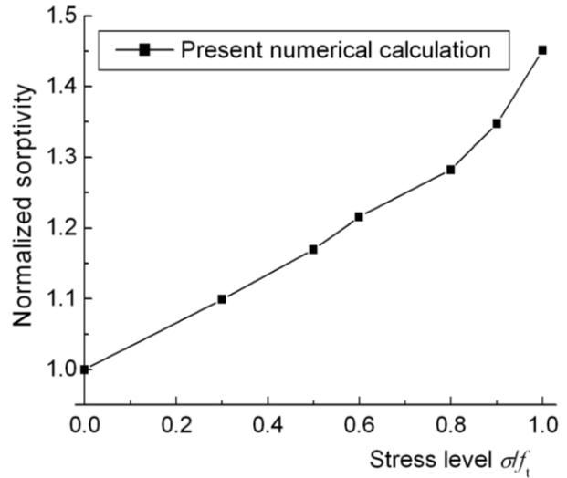
Fig. 10 Effect of compressive stress level on the sorptivity and comparison with test results
