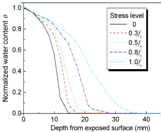
Fig. 11 Water content distribution under different compressive stress levels
