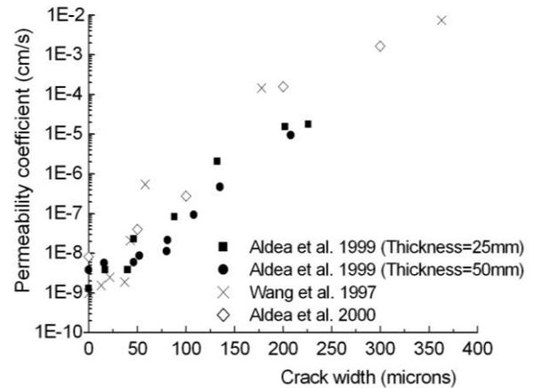
Fig. 2 Cracking effect on permeability of concrete
