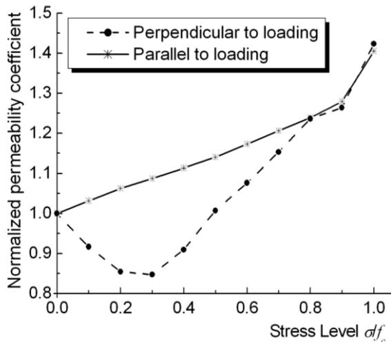
Fig. 7 Results of water penetration direction on the permeability coefficient
