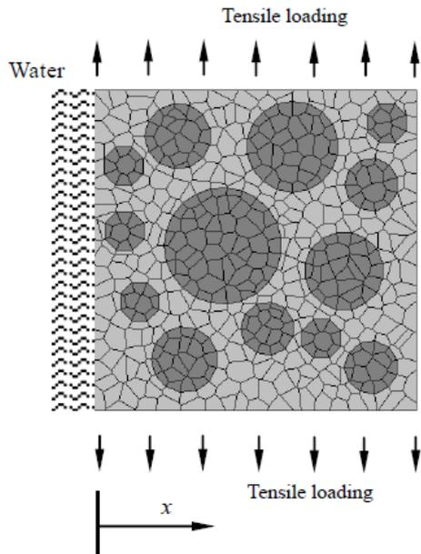
Fig. 9 Analysis conditions of the specimen under tension
