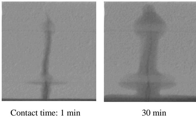
Fig. 1 Water penetration into a single crack
