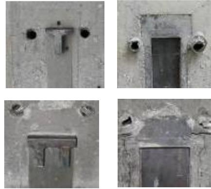
Fig. 5 Shear bracket and beam socket after tested
