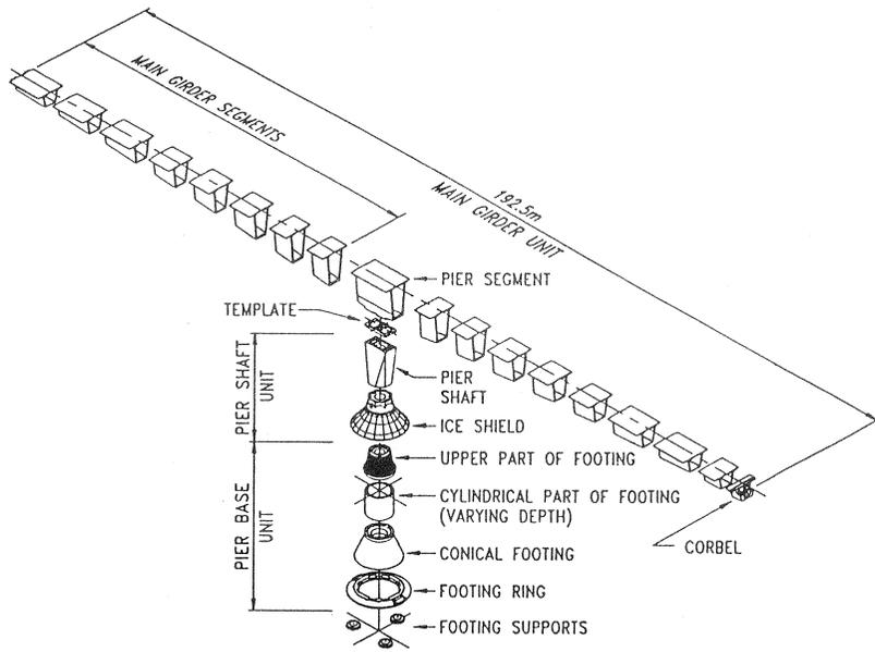
Fig. 11- Segmental components of the prefabricated units
