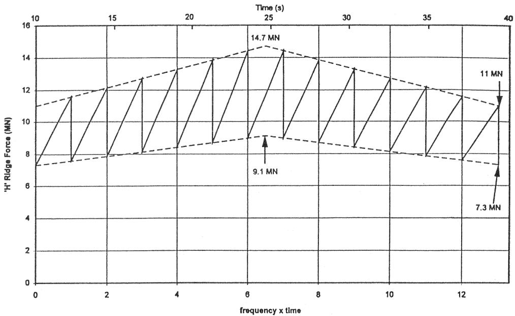
Fig. 7- Idealization of the variation of the horizontal component,  $H$  of ice force on a pier in the marine spans. The scale on top edge of the figure is used for a pier whose lowest natural frequency = 0.44 Hz. (Note the initial starting time is selected at 10 s.)
