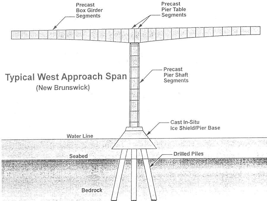
Fig. 10- A pier and a balanced cantilever built in segments. The part shown represents typical part between centre lines of adjacent spans, each of length 93 m of the bridge approaches
