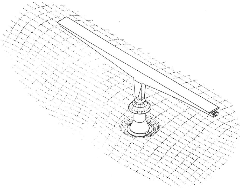
Fig. 21- A pier with two overhangs ready to receive the drop-in units
