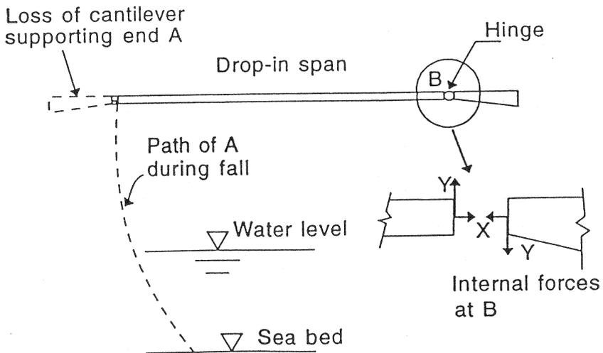
Fig. 8- Definition of the internal forces at a plastic hinge developed at B in an accident in which the support at A of the drop-in unit is lost in the structural system shown in Fig. 3b.
