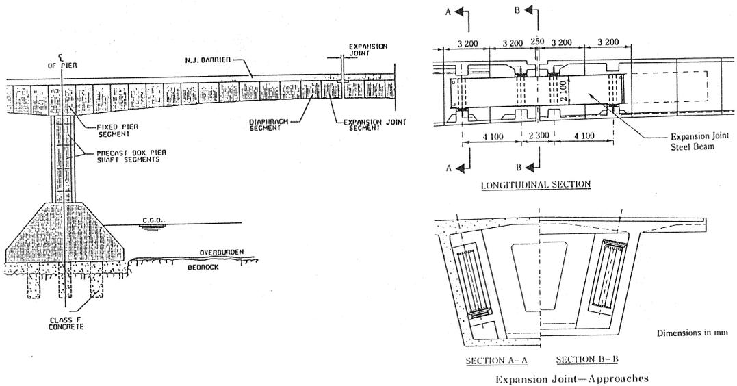
Fig. 10\*- Expansion Joint - approaches
