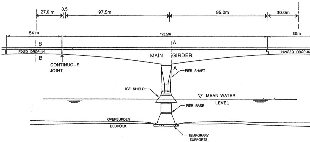
Fig. 4- Elevation of a typical pier and two halves of marine spans
