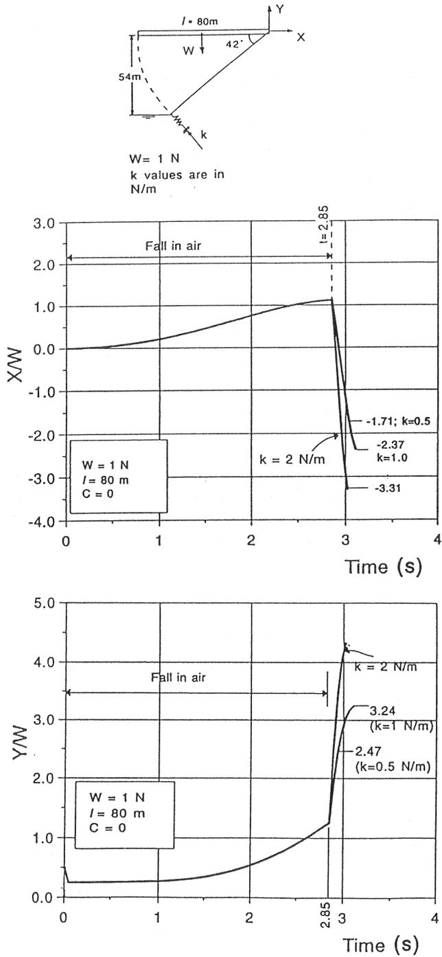
Fig. 9- Variation of the forces X and Y at the right-hand hinged end of a beam, when the left-hand end is allowed to fall down on a spring with varying stiffness.
