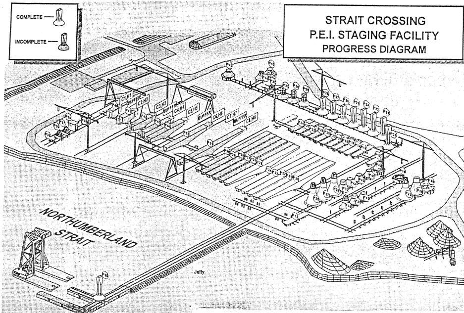
Fig. 20- Pictorial view of the precasting yard at 144 weeks after the beginning of the project (October 1993)
