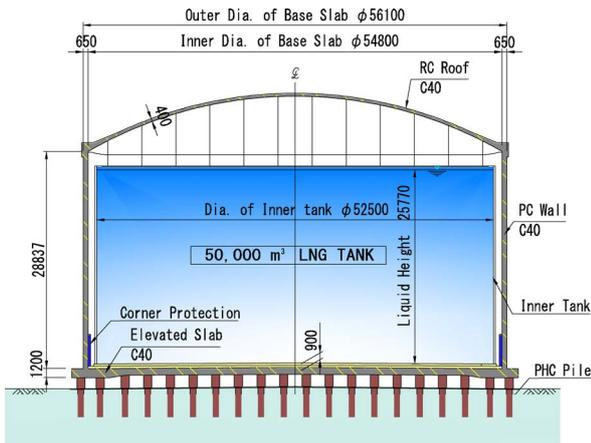
Fig.3 Dimension of 50,000m<sup>3</sup> PCLNG Tanks
