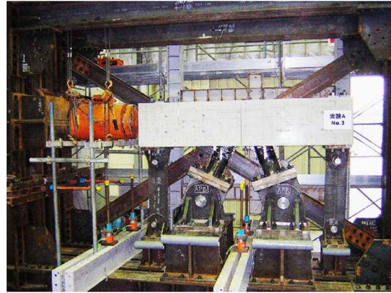
**Fig.6 Loading test of new panel point**
