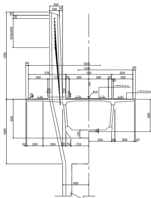
Fig.3 Cross section
