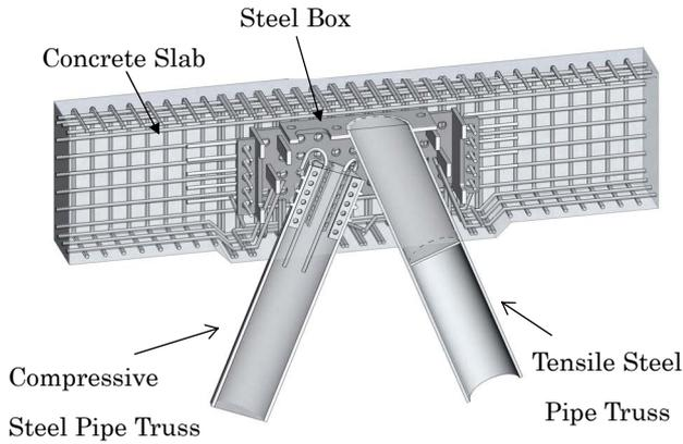
**Fig.5 Structure of new panel point**
