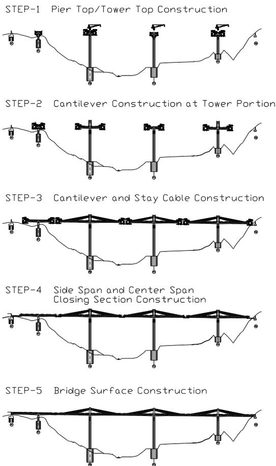
**Fig.7 Construction steps of superstructure**
