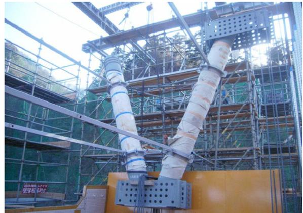
**Fig.9 Fixed steel pipe truss**
