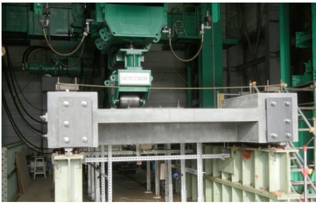
Fig.2 Wheel load running test in progress
