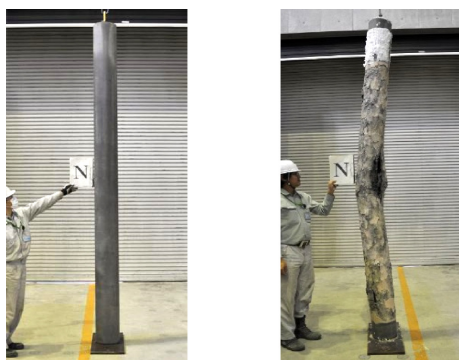
Fig.3 Specimen before (left) and after (right) fire resistance test
