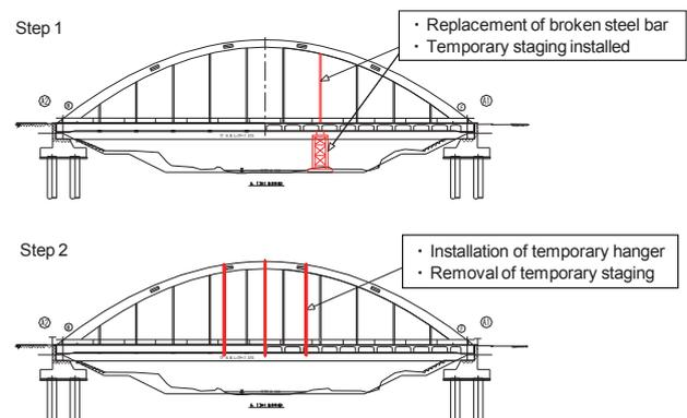
Fig. 4 Outline of emergency repairs
