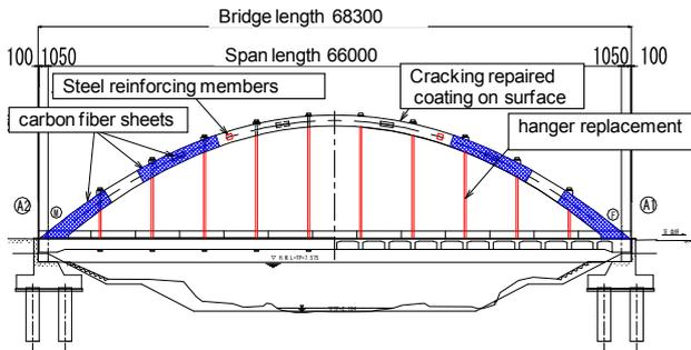
Fig. 5 Outline of permanent repairs
