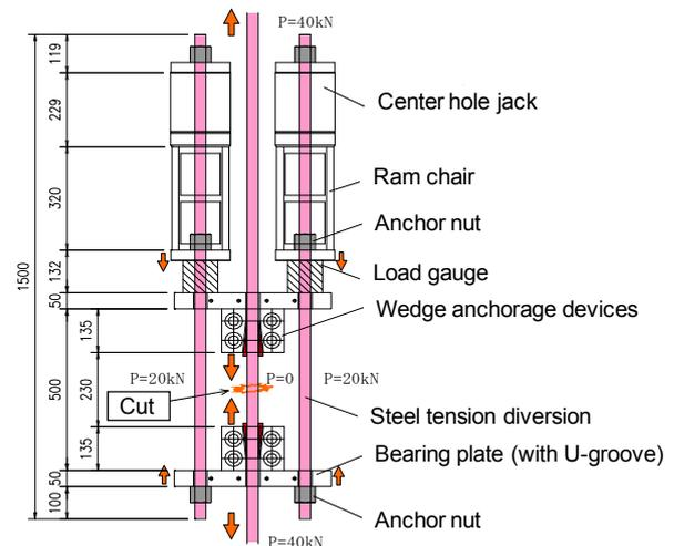
Fig. 7 Tension releasing equipment
