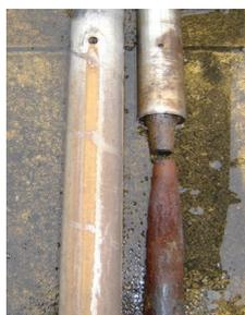
Fig. 2 Broken steel bars
