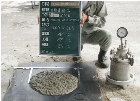
**Fig.5** Concrete with slump flow of 50 cm
