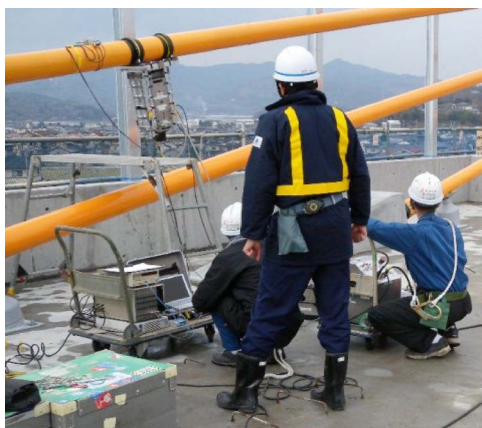
Fig.6 Vibration test for stay cable
