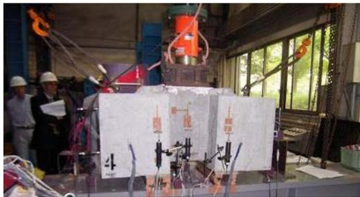
Fig. 8 Double shear test
