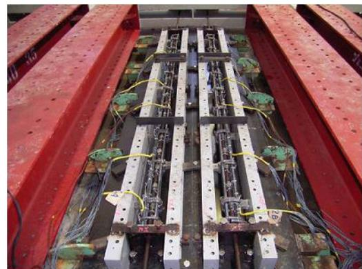
Fig. 9 Test specimens (before placing concrete)
