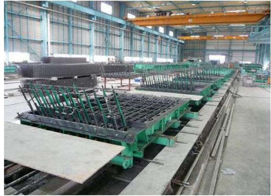
Fig. 11 Manufacturing of the PPWs
