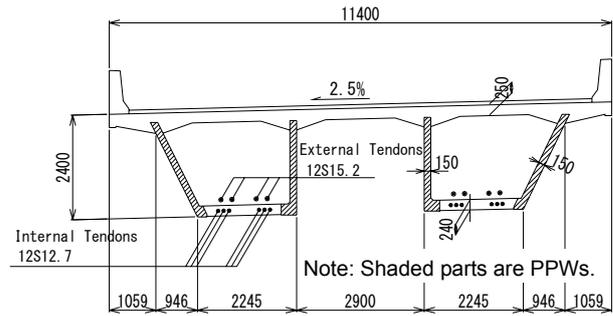
Fig. 3 Girder cross section
