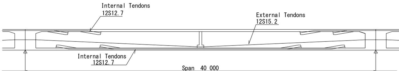
Fig. 6 Tendon arrangement
