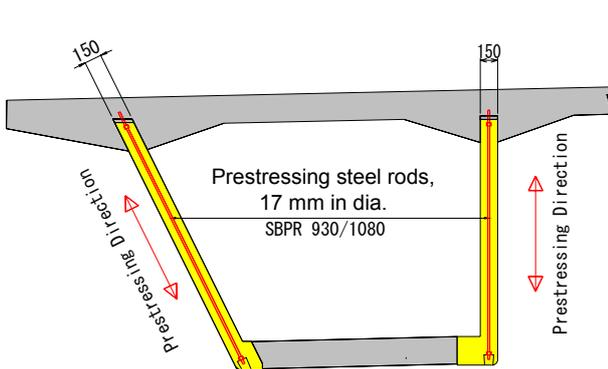
Fig. 4 PPW cross section
