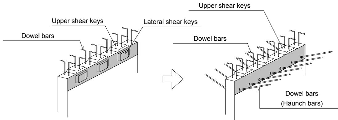
Fig. 7 PPW joint structure
