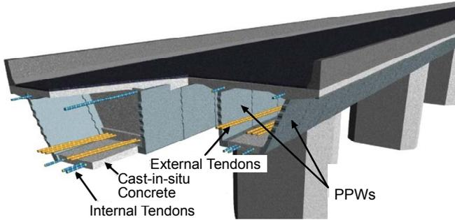
Fig. 2 Perspective of the main girder
