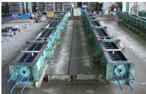
Fig. 7 Steel bar arrangement of RC struts
